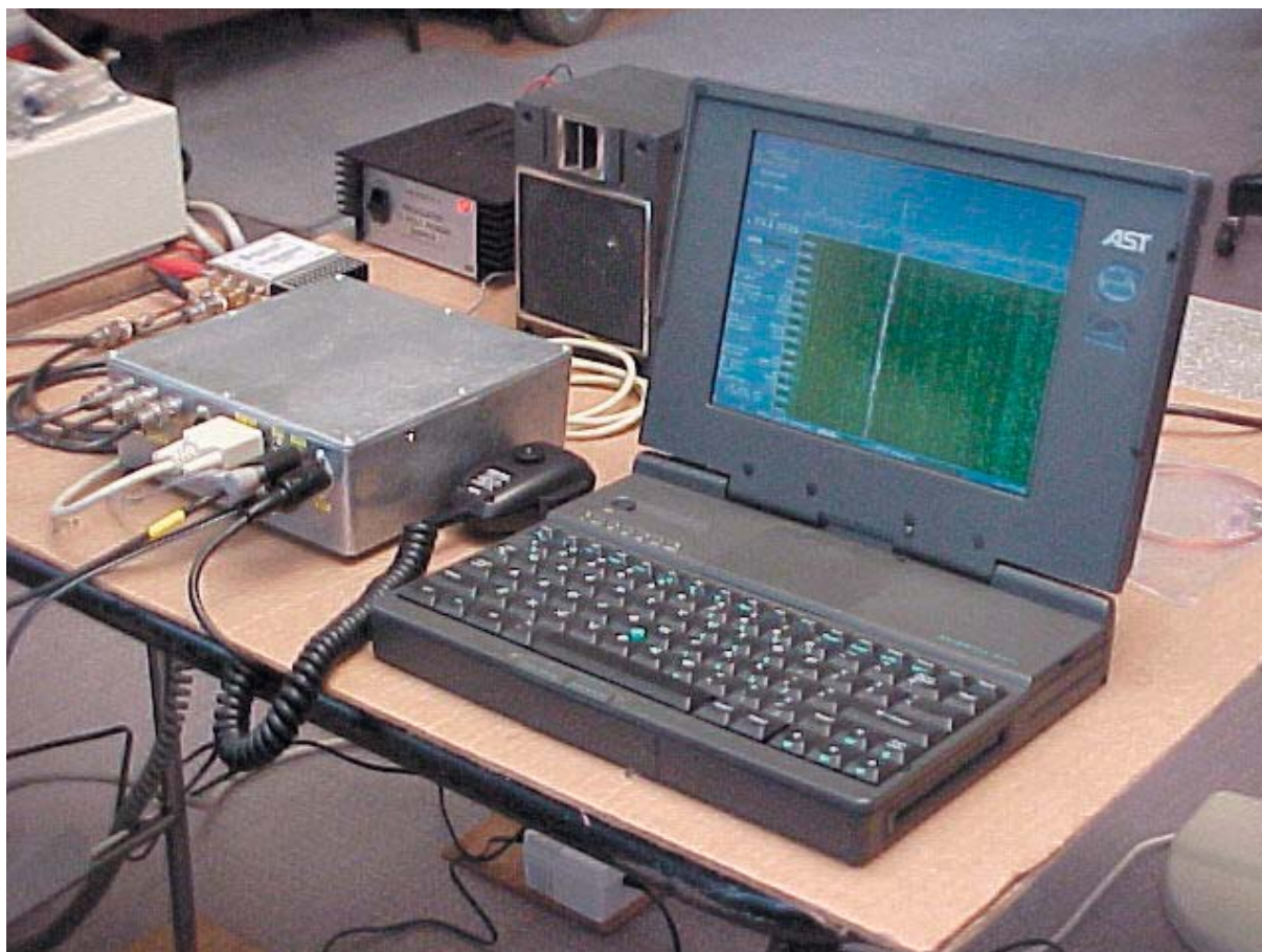
Figure 1 The DSP-10 setup used by W7LHL. The aluminum box to the left of the laptop computer has the DSP board, RF and IF hardware. The laptop computer is a front panel and control device for the station. Displays on the computer show the spectrum of the received stations and the processed results from the weak-signal modes, such as PUA43. (Photo by W7SLB)
